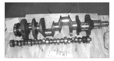
This is the same camshaft I use in my 1929 Ford Roadster. This camshaft works well with automatic transmissions as well as with power boosters. The crankshaft and flex plate are toast, they appear to have suffered from some sort of side force that caused the wall next to the number 6 connecting rod to become gouged out and the flex plate to be deformed, both will be replaced.
