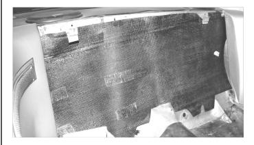
I am installing a reinforcing brace behind the rear seat to help stabilize the rear structure of the car, which would be subject to being over-stressed by the front end improvements if nothing is done.
