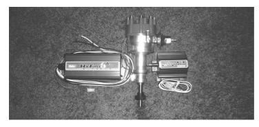
I am replacing the distributor and coil with Mallory units as well as a microprocessor control box.
